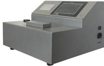
YT-SCT500 Short Span Compression Tester is a new type of instrument researched and developed according to the requirements of international standard ISO 9895 and national standard GB/T 2679 · 10 《paper and cardboard short-distance compression test method》 .
